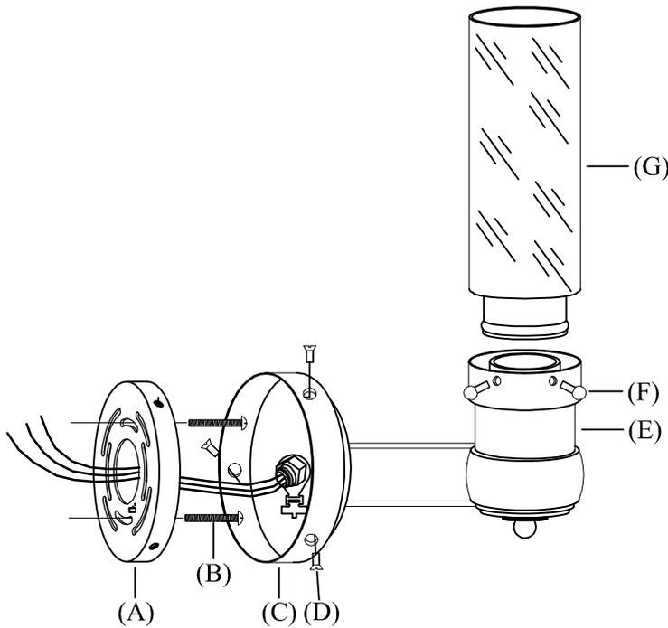
1. Attach ground (green) wire to ground wire from wall outlet box (usually green or copper in color), fasten together with a plastic wire connector. Tightly wrap the wire connector with electrical tape so the end of the connector is sealed.
