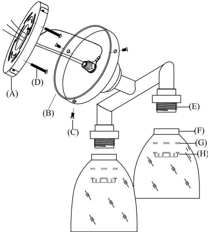
1. Attach the ground (green) wire to the ground wire from the wall outlet box (usually green or copper in color), and fasten together with a plastic wire connector. Tightly wrap the wire connector with electrical tape so the end of the connector is sealed.
