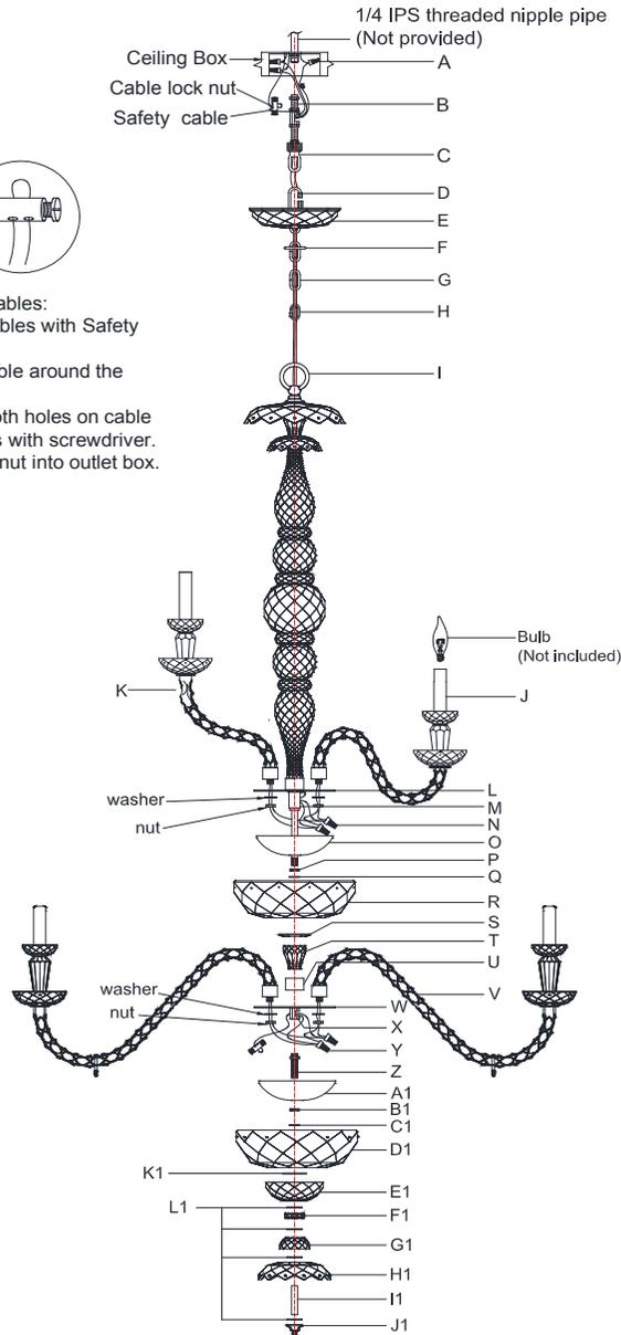
12. Attach plastic washer (O) & crystal bowl (R) & crystal (S) & crystal (T) go through the threaded nipple (M) and secure with connector (U).
